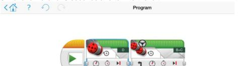
Instruction: "How could we change the direction of the car with Move Tank? Could we change the direction by manipulating the speed of two wheels? Expected Answer: We could change the speed of each wheel to control the direction. Example:
